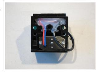
Drill a hole in turn signal housing and route wire directly inside to leave no exposed wire.
